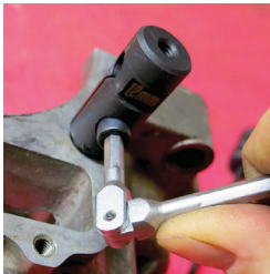
Maximum torque for 6 mm bolt is 7 lb/ft
